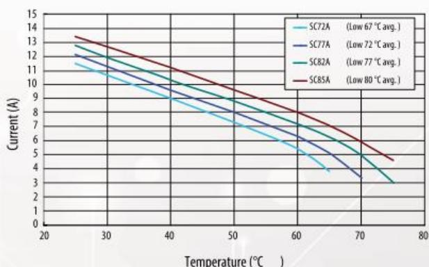
Ambient Temperature Impact on Mini-breaker Operating Currents
