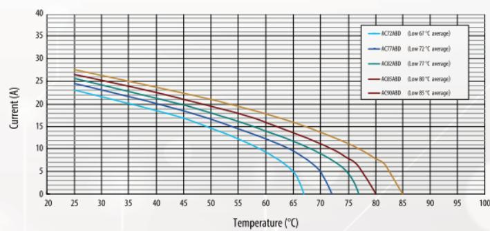
Ambient Temperature Impact on Mini-breaker Operating Currents
